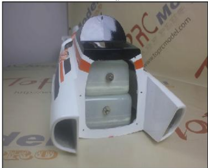
27. Put the fuel tanks in the fuselage.
